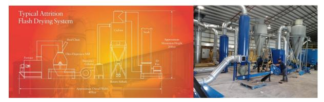
IEC Thermo HEMP dryers combine established drying and processing techniques into an attrition flash drying process that keeps cannabinoid molecules intact and undamaged, providing a timely and cost-effective means of stabilizing your valuable harvest before mold, mildew or composting can occur, allowing for future processing at a pace you determine.
